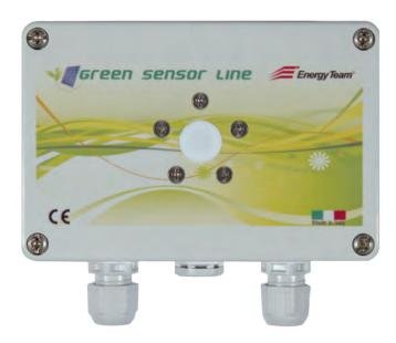
The composite sensor of this solarimeter can detect solar irradiation and temperature and send the data to a data logger through its outputs than can be either set as digital pulsed or analogic (4-20mA). The sensor allows precise detection of two fundamental parameters to evaluate the performance of photovoltaic plants: irradiation and panels' operating temperature.
