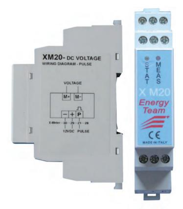
The XM20 device reads a continuous analogical voltage signal up to 1000VDC and converts it into a 0-5 Hz pulsed signal compatible with the standard input signals for CM2 Solar or XRWU GOLD/X-Meter. Guaranteed precision of 0.5% of full scale.
