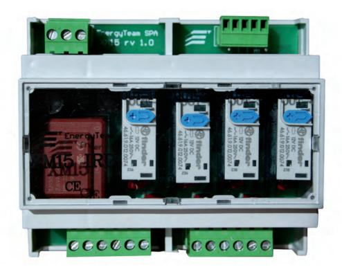
The X-Meter counts 4 ON-OFF output activators to manage 4 outputs with 24Vac/Vdc maximum voltage and 100mA maximum current. These outputs must be interfaced with an XM15 module to manage standard loads in a 220Vac single phase network.
